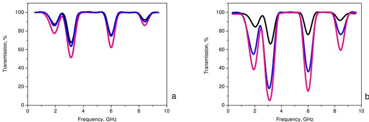
**Figure 2.** Influence of the illumination geometry in: (a) uncoated cell and (b) SC-77 coated cell without illumination (black), with one-side illumination (blue) and with homogeneous illumination (pink).
