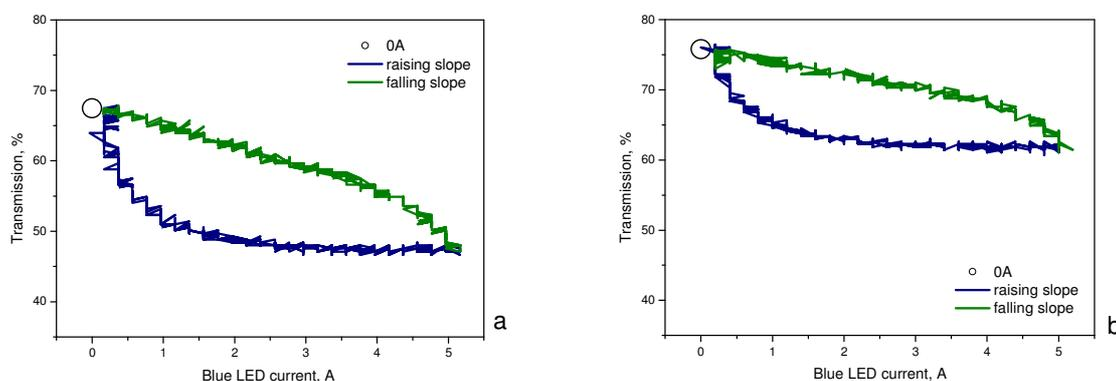
**Figure 4.** Transmission as a function of the blue LED illumination intensity and the direction of its tuning at 0.2 Hz and 4- $\mu$ W 780-nm laser light in an uncoated cell.
